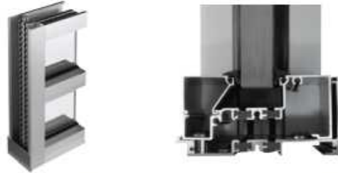
Trifab™ 451UT uses a dual Isolock™ thermal break (right) and features a new high-performance sill design, which incorporates a screw-applied end dam (left), ensuring positive engagement and tight joints between the sill flashing and end dam.
